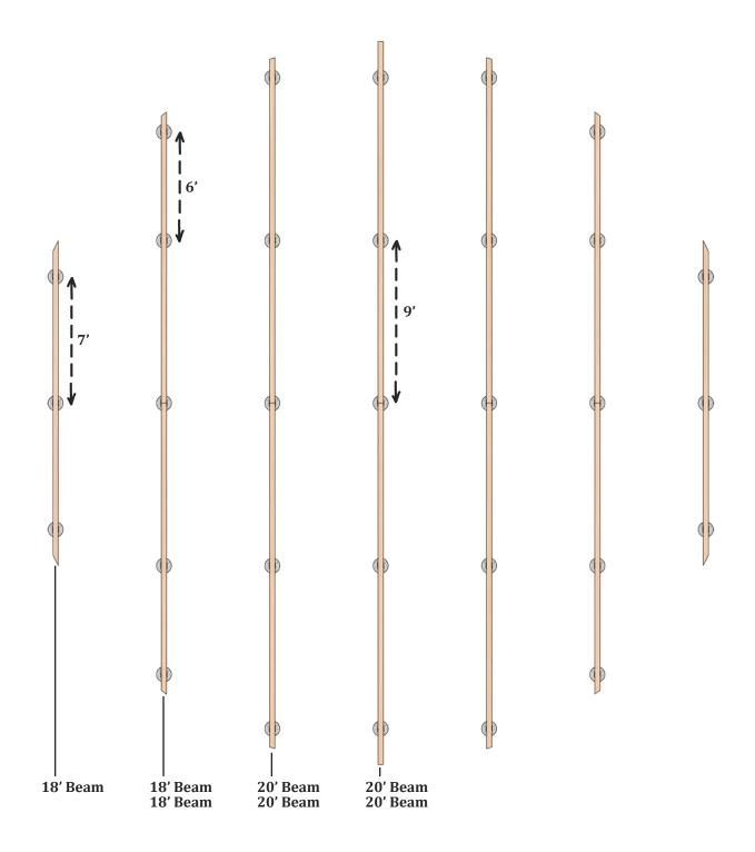
\*Diagrams show ideal beam length based on materials list quantities. Start your layout from the middle. Perimeter cuts as shown in the diagram can be made after laying plywood.
