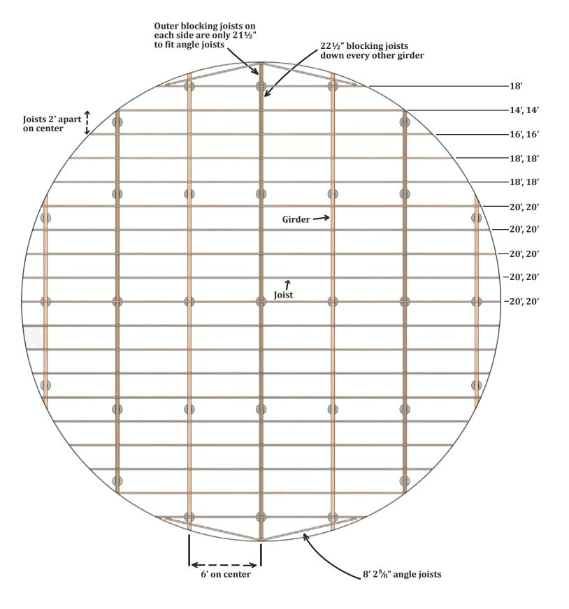
\*Board lengths in the materials list are intended to be the most efficient sizes for minimum excess. Use the closest length for each main joist, and cut the rest for blocking. If some board lengths are unavailable at your location, adapt the design as necessary as long as each joist is secured at two or more locations.
